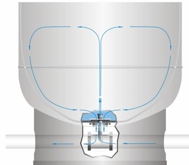
Flow-Thru technology assures total recirculation of the tank's water content.
